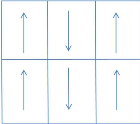
7. Lay the rolls to provide as few seams as possible with economical use of materials. All rolls being installed on a given day must be unrolled the day before and allowed to relax overnight.
