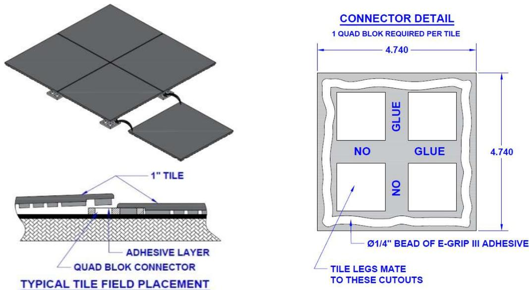
Note: Adhesive spills must be removed while still wet. Use a dry rag to pick up the majority of the adhesive. Wipe the remaining residue with a rag dampened with mineral spirits, followed by a rag damp with water to remove the mineral spirits. Cured adhesive can only be removed from surfaces by mechanical means, such as scraping or sanding.
