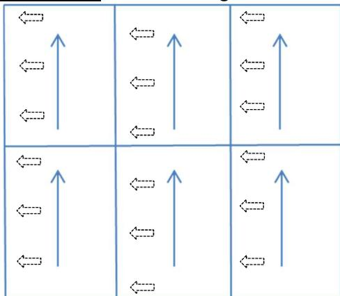
7. **PLEASE NOTE: Wood board pattern rolls have partial board widths on each side of the roll from the factory; factory edges are suitable for installation. If removal of these partial board widths is specified, material yield will be reduced on the job and should be taken into account when estimating.**
